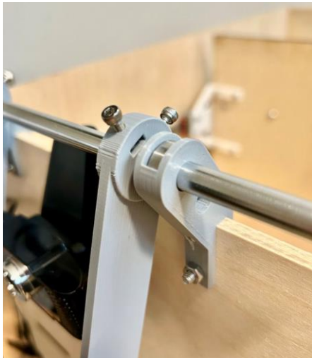
Figure 24: Fabricated hub for Lifting Arm and Wheels
